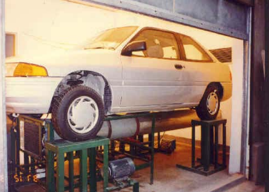
Automotive air conditioning controller and test bed
